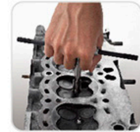
1. Tap re-drilled hole using tap
