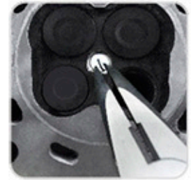
5. Using Pliers, take off pin on insert
