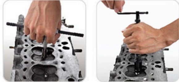
1. Tap re-drilled hole using tap
